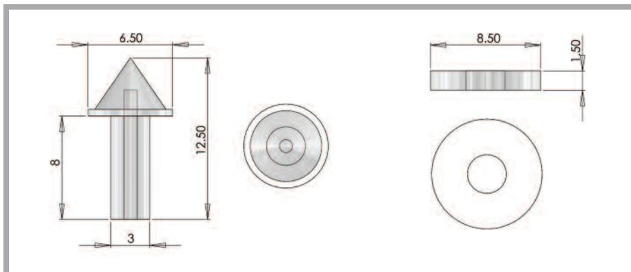
Small conical fittings made from polycarbonate for star effects. Supplied with back washer which can be optionally fitted.
