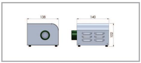
The UFO Mercury light source is a powerful, yet efficient fibre optic light source, powered by LED technology.
