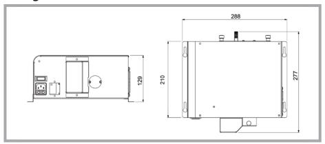
A low profile light source which uses either a 70W or a 150W metal halide discharge lamp to give much greater brightness than those powered by halogen lamps.
